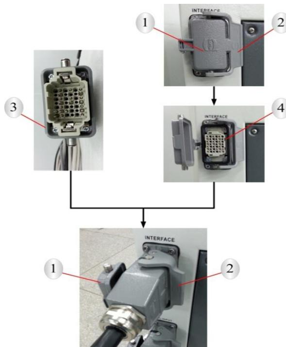
1. Protective Cap; 2. Locker; 3. Plug; 4. Socket
