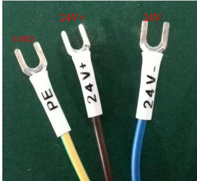
Figure 3. Definition of power line wires
