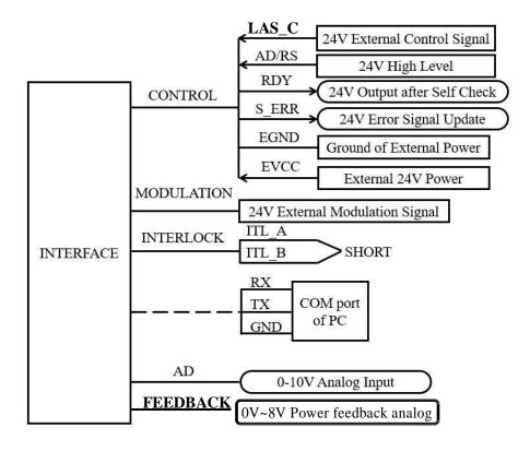
Figure 19 Wiring in RS-232 Mode
