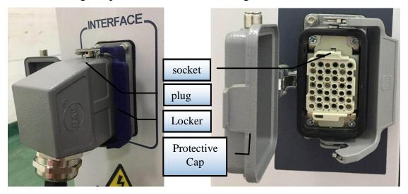
Figure 13 Control port and socket on the lock.
