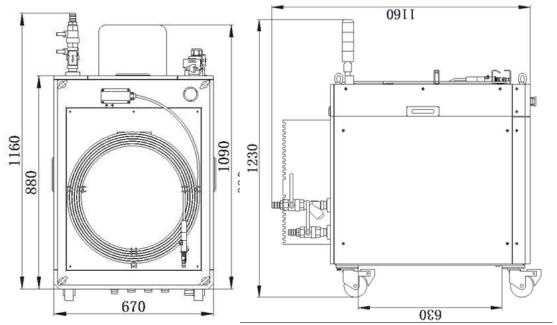
Figure 1-b Top and left view of the laser.
