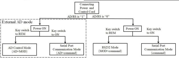
Figure 14 The process of entering a control mode.
