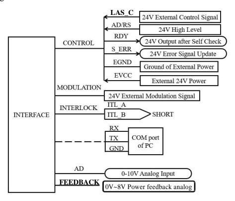
Figure 20 Wiring Diagram in AD mode.
