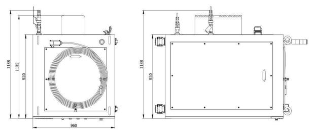
Figure 4-b Top and left view of the laser.
