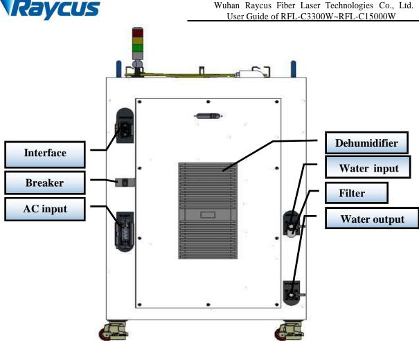
Picture 9-d Rear view of C15kW product panel.
