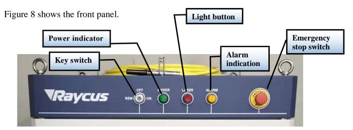
Figure 8 Front view of the panel.
