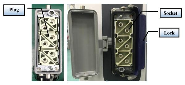
c) The picture of 15kW power port plug / socket.
