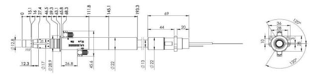
Figure 5 RFL-QBH output optical cable head
