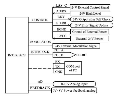
Figure 15 Wiring of Serial Port Communication Mode
