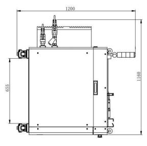
Figure 3-b Top and left view of the laser.
