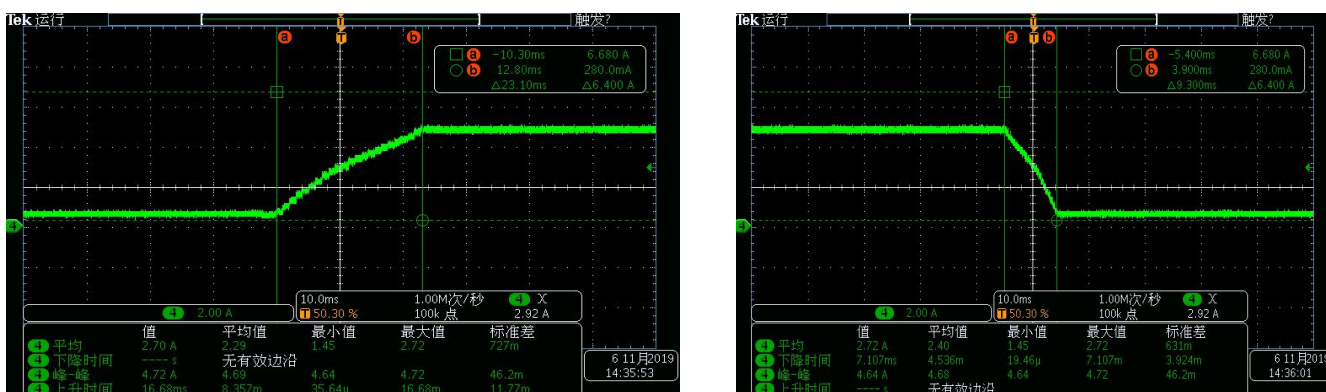
Figure 39 The power slow rise and fall setting area interface and measured programmings
