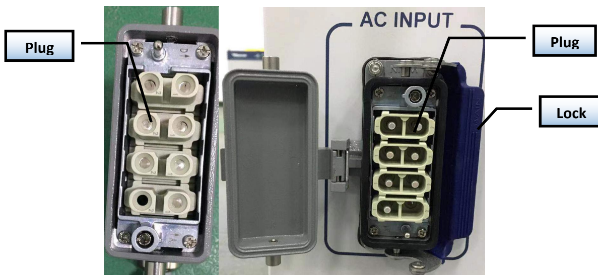
Figure 17-b RFL-C6000XZ physical picture of power cord plug and socket
