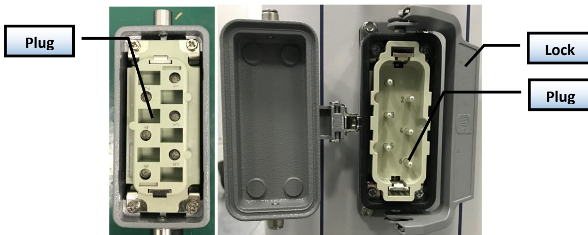
Figure 17-a RFL-C4000XZ physical picture of power cord plug and socket
