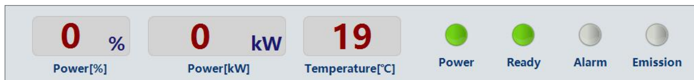
Figure 34 A diagram of the laser's main display area
