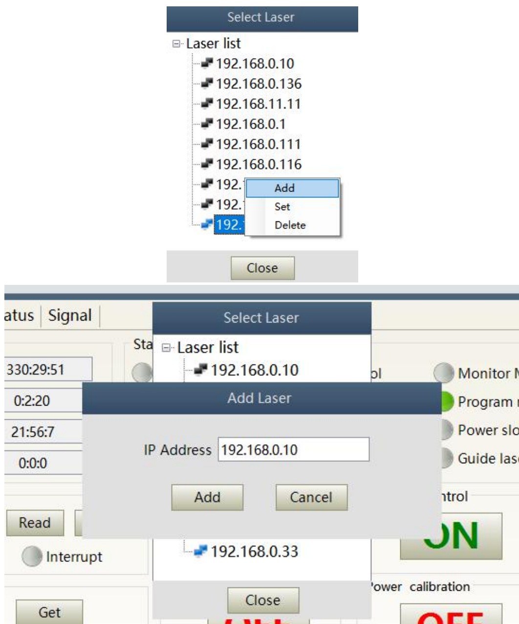
Figure 32 Procedure for adding a laser to the PC software
