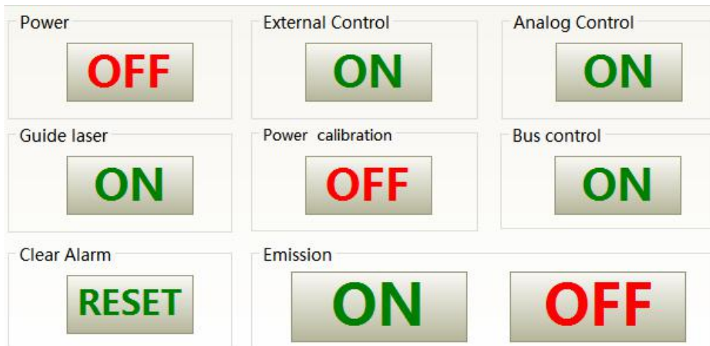
Figure 37 Laser power-on, mode selection, light out control display area
