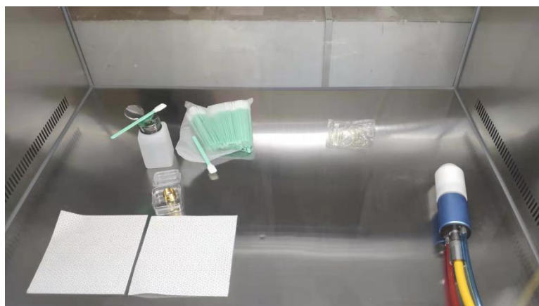
Figure 10 The output optical cable placed in the clean bench with the ventilation turned on
