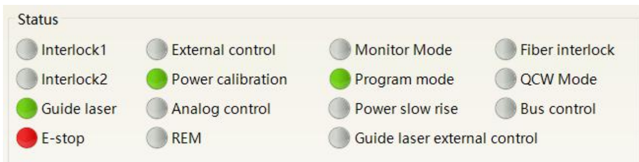
Figure 36 A diagram of the laser's working status display area
