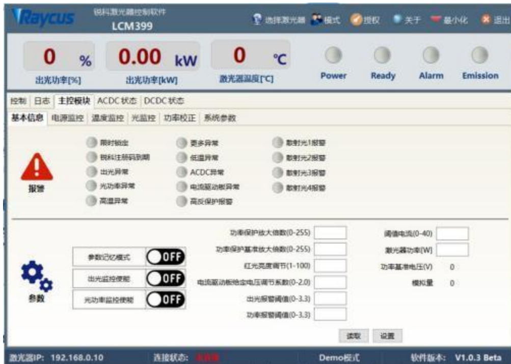
Figure 16 Main control module status information interface
