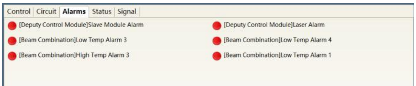
Figure 38 Laser alarm type display area interface
