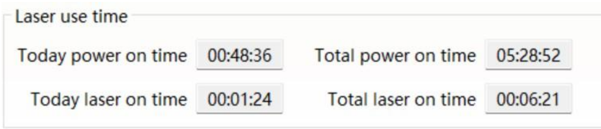
Figure 32 Display menu for accumulated working time of laser
