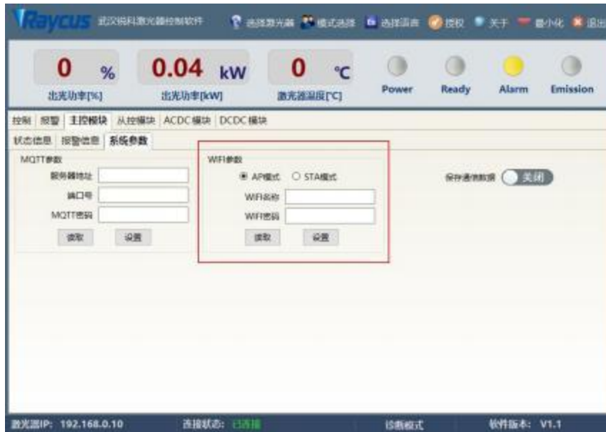
Figure 18 Main control module system parameter interface
