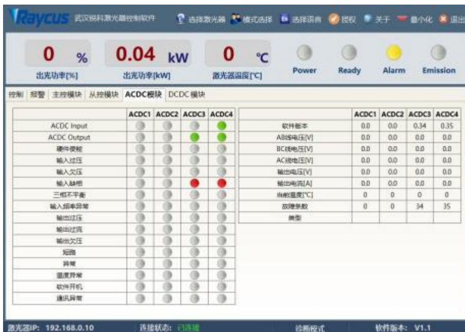
Figure 21 ACDC module interface
