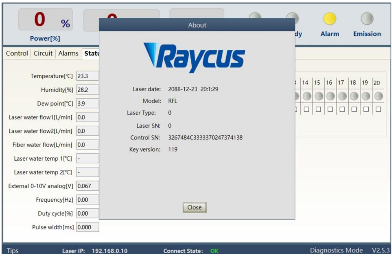
Figure 44 Laser relevant information query interface
