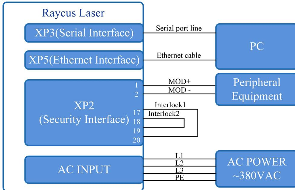
Figure 20 Wiring diagram of external control laser emission in programming mode, in ON mode
