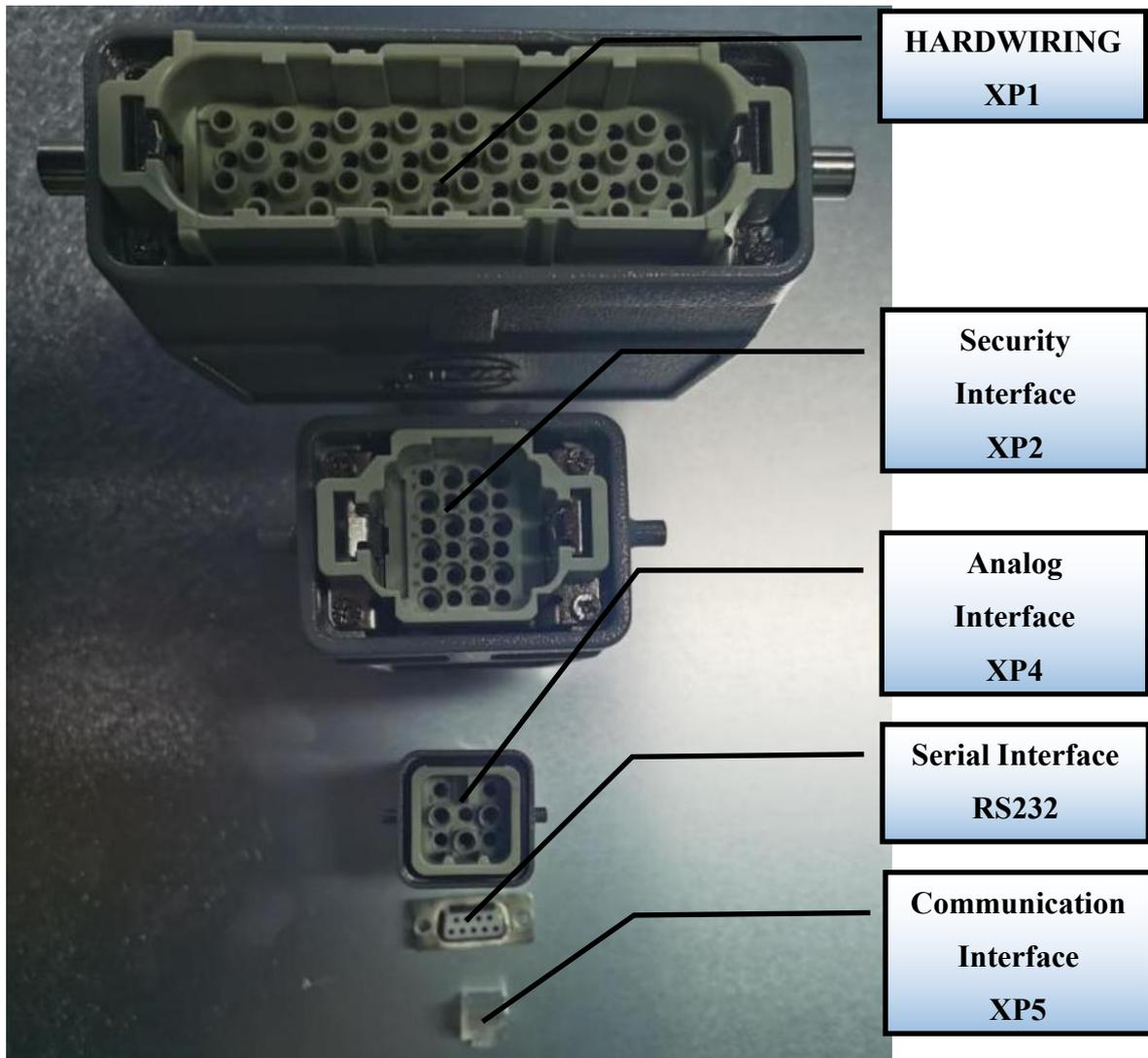
Figure 15 Control signal line
