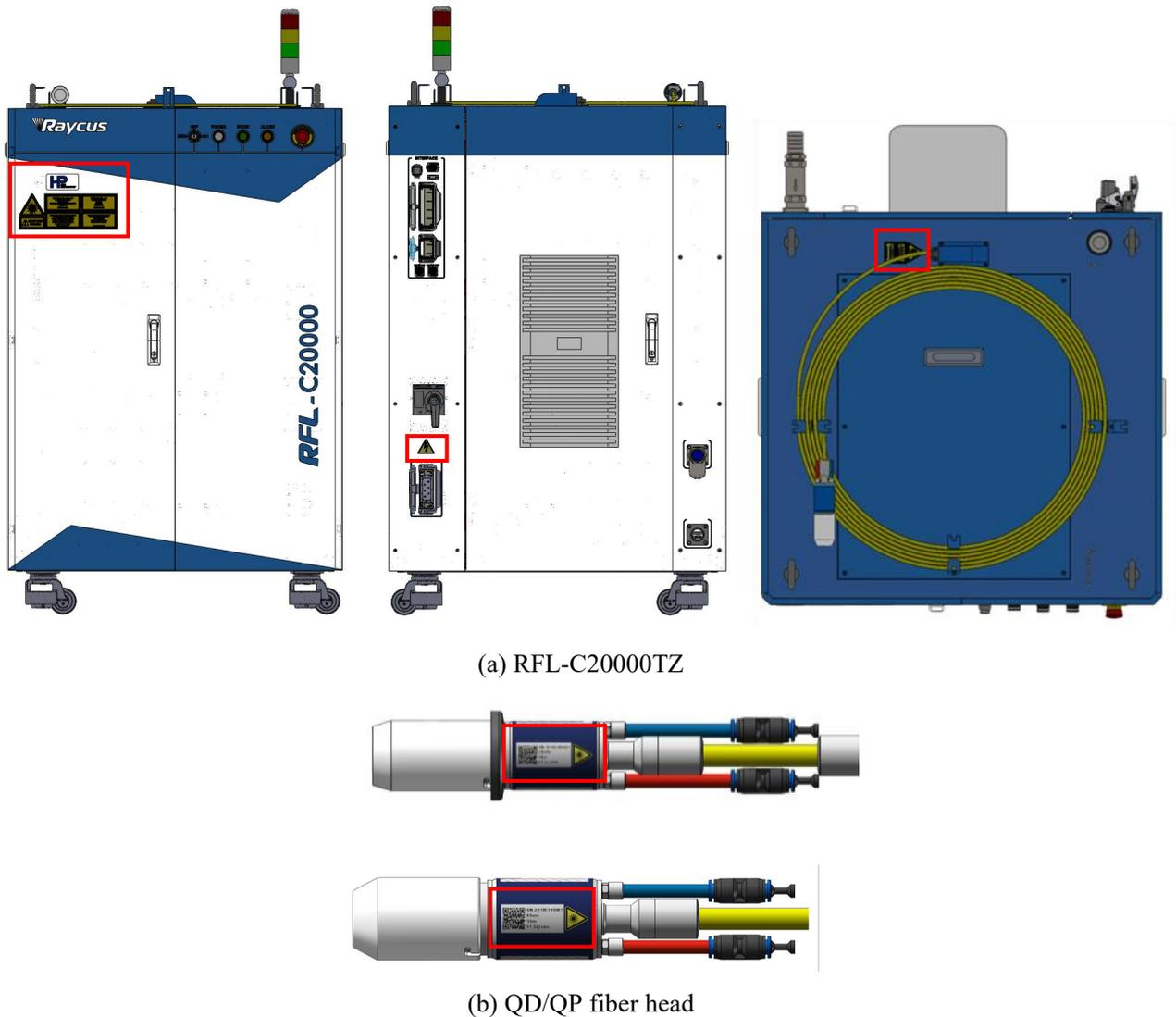
Figure 1 Schematic diagram of the distribution location of laser safety signs
