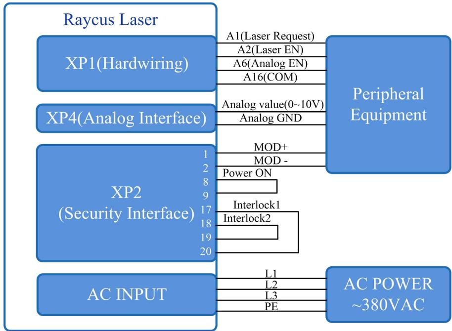
Figure 21 REM mode power and laser emission are externally controlled wiring diagram
