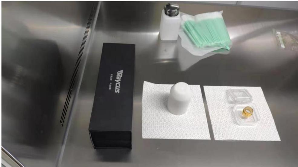
Figure 9 Accessories that customers need to keep: black protective box, white dust cover, type A end cover
