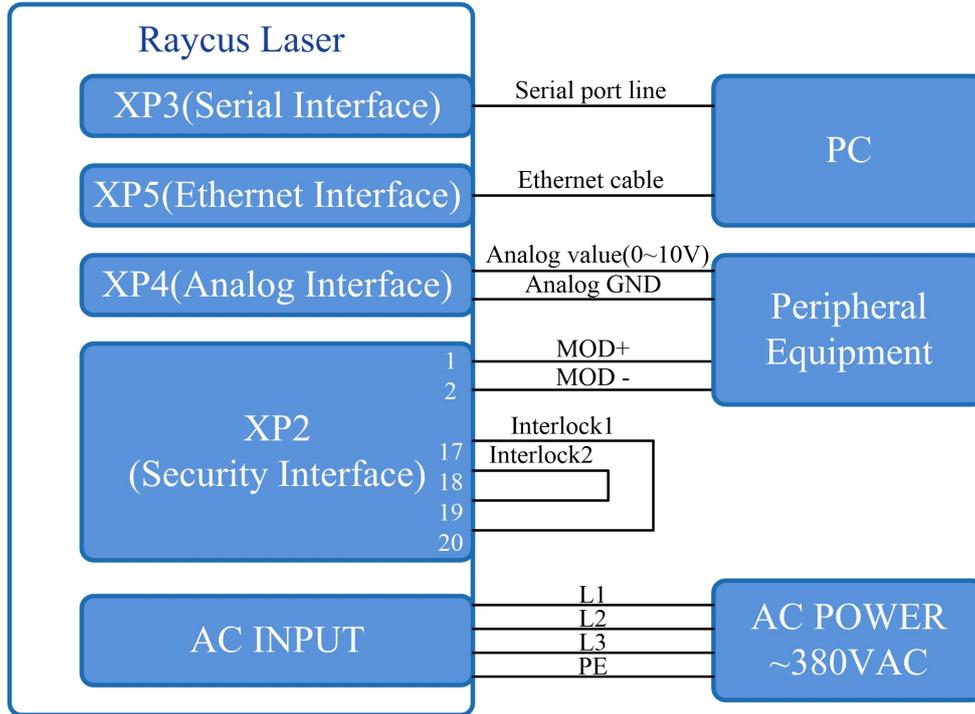
Figure 19 In ON mode, the wiring diagram of the power and laser emission controlled by analog signal
