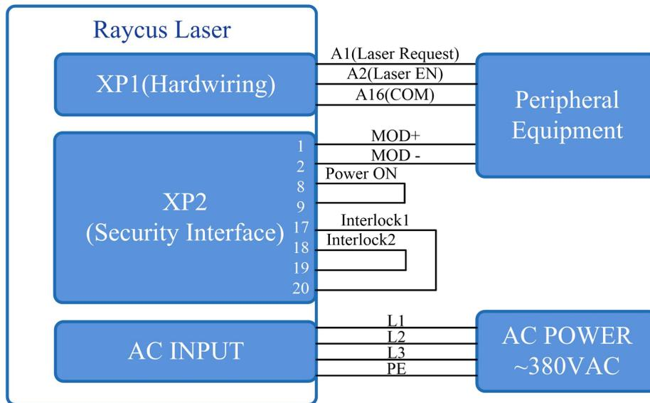
Figure 23 Wiring diagram of power internal control and laser emission external
