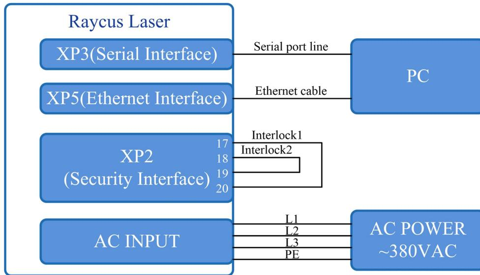
Figure 17 Software mode wiring diagram when key switch at “ON” position
