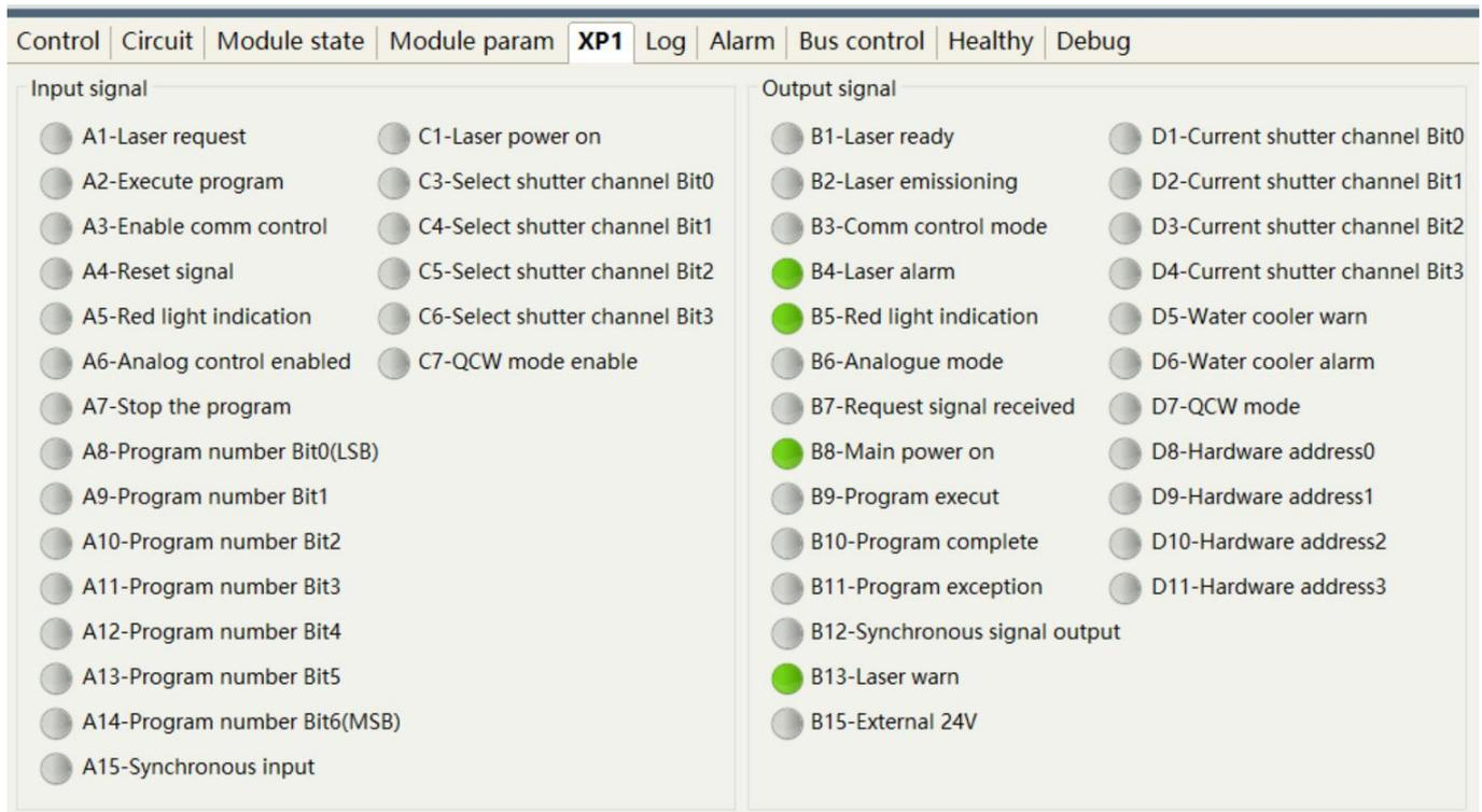
Figure 45 The interface status in diagnostic mode
