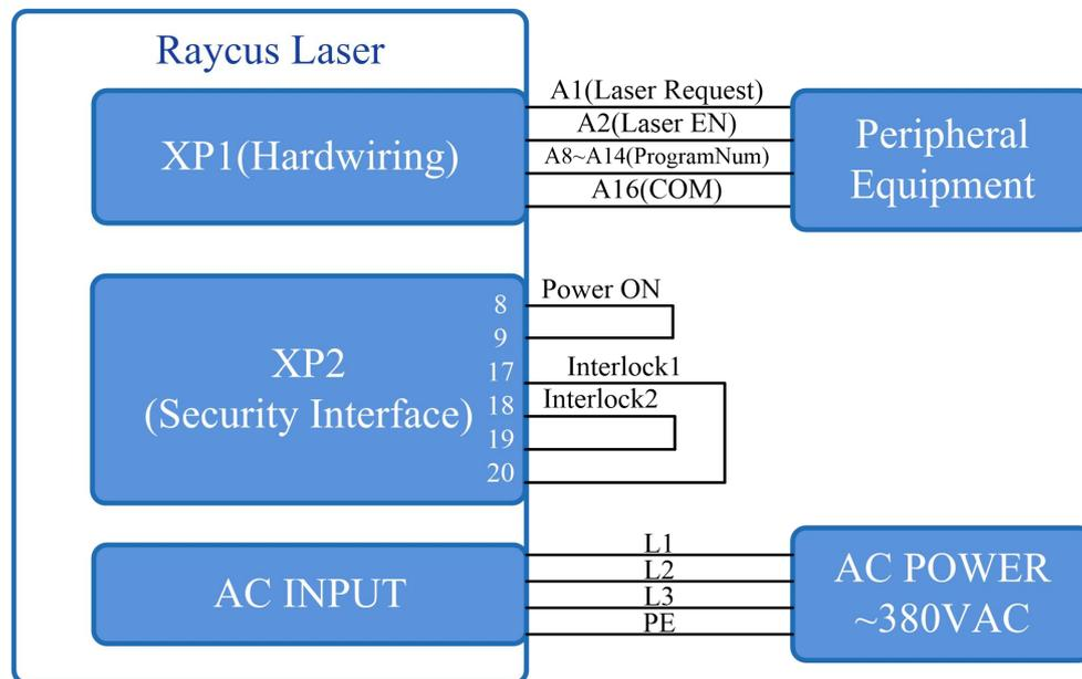
Figure 24 Wiring diagram of programming mode in REM Mode
