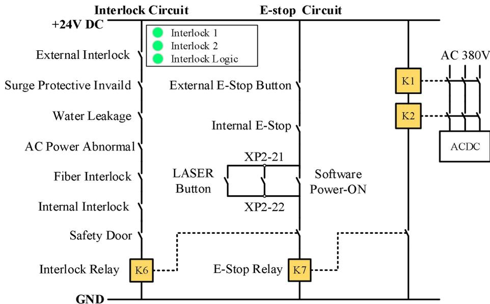
Figure 16 Schematic diagram of the internal electrical circuit of the laser
