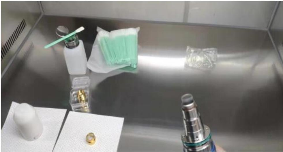
Figure 8 Remove the A -type end cap on the optical cable
