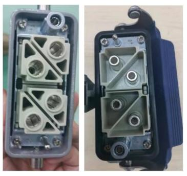
Figure 14 Pictures of power cord plug and socket of 15kW/20kW laser
