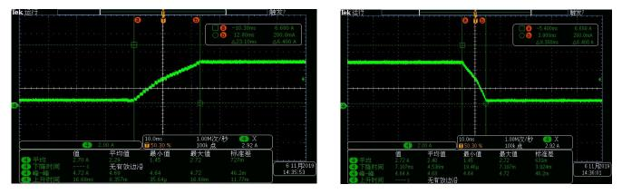
Figure 36 The power slow rise and fall setting area interface and measured programmings
