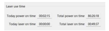
Figure 32 Laser cumulative operating time display interface
