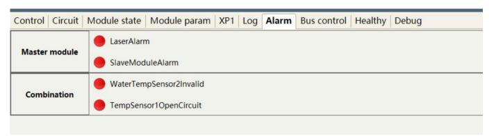
Figure 39 Laser alarm type display area interface
