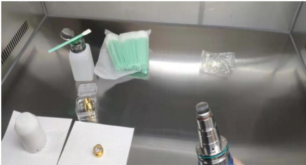
Figure 10 Remove the A -type end cap on the optical cable
