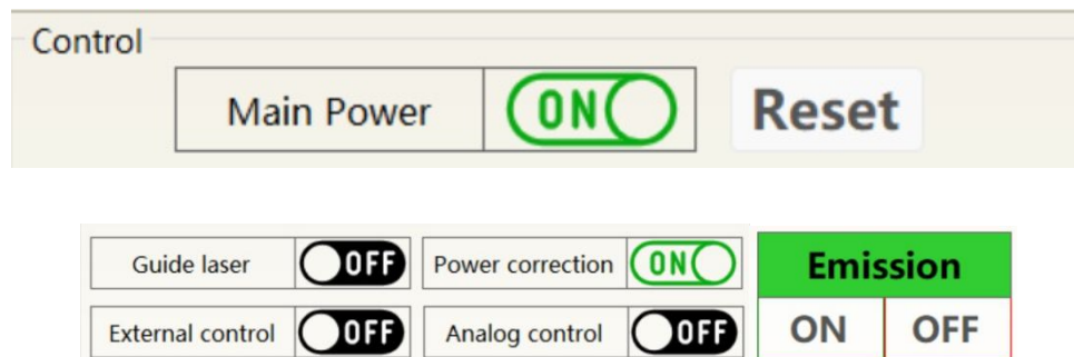
Figure 34 Display area for laser power on, mode selection, and light output control
