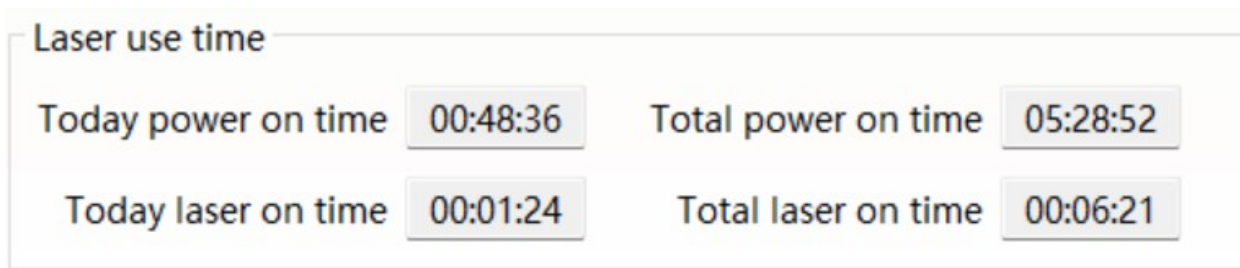
Figure 33 Display menu for accumulated working time of laser
